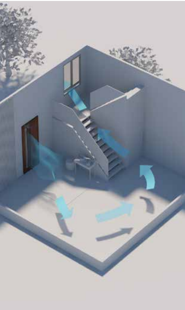
Provide passive ventilation environment
